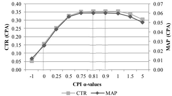
**Figure 5: CTR and MAP scores for CPA with various CPI  $\alpha$ -values. MAP<sub>max</sub> at  $\alpha = 0.81$ , CTR<sub>max</sub> at  $\alpha = 0.9$**
