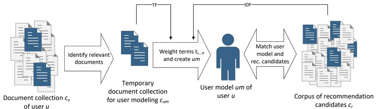
Figure 1. Document recommendation and user modeling process with TF-IDF and TF-ID<sub>u</sub>F
