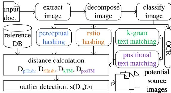
**Figure 2: Overview of adaptive image-based PD approach.**
